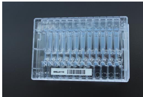
bottom bar code – scanned by the instrument nest
