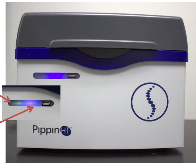
Figure 4.2. Instrument indicator lights and optical array.
