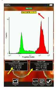
The Moxi V<sup>™</sup> provides particle concentration and precise sizing information for each gated region, total counts information, fluorescent percentages, and median fluorescent intensities (all where applicable based on the channels selected) for each test. Two example test view screens are shown above (left to right: Fluorescence vs. size scatter (dot) plot, Single Channel Histogram Display).
