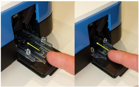
4. Once the insert is all the way in, try closing the cassette door. If insert is properly installed, door should close all the way. If the door doesn't close, try to push the insert further in.
