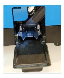
2. Gently lift up on the center tab (red arrow in images below) of the tray insert while pulling out to slide the insert out. Pull insert all the way out. (Refer to images below)
