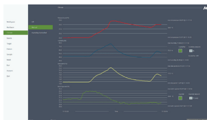
Climate Control: Humidity and Dew Point Control with a CV of 1%
