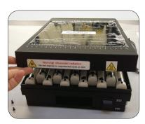
Using a pair of needle nose pliers with grip as an aid, rotate the bulb and lift it out of the ballast housing.
