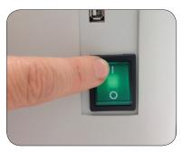
• **Turn on the Tablet Power.** The tablet power is located at the top of the tablet. Press and hold the button to turn on the tablet power.
