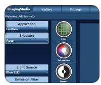
Select Blue LED under Light Source, Orange Filter under Emission Filter, Gel Tray under Tray Type, and Gel under Aperture Type. Name the application and select Save.
