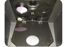
Remove the old filter and screw in the new filter.
